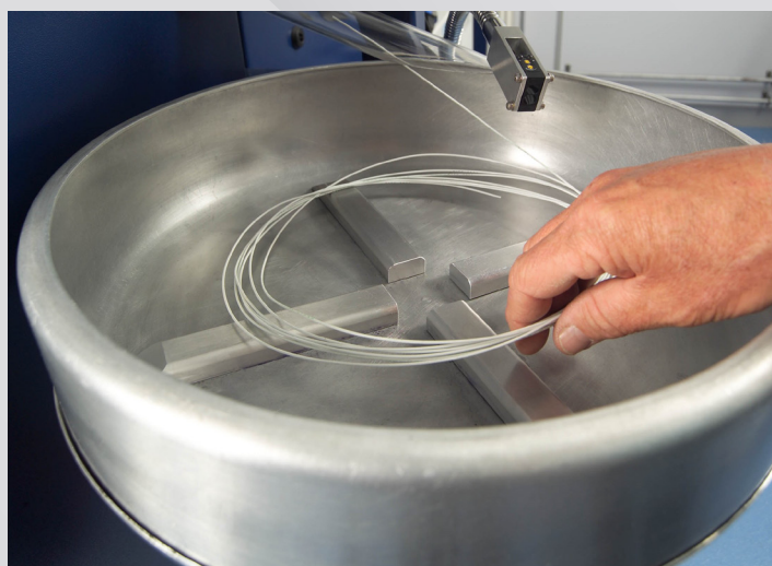
above: coil pan with coil pan sensor
